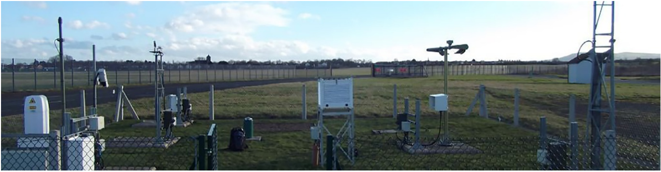
FIG. 2.2 Example of a ground station-based observation part of the UK Met Office (UKMO) “HadUK-Grid” surface monitoring network (see also Fig. 2.3 for wider network of ground station-based observations). The instruments are generally located in an open field away sufficiently far from any potential artificial influence or obstructions that can contaminate measurements, e.g., turbulence from roadside traffic/airport runway, shadow of a building structure, etc. Image from HadUK-Grid—UKMO ( https://www.metoffice.gov.uk/research/climate/maps-and-data/data/haduk-grid/haduk-grid ). Readers are also guided to http://www.jma.go.jp/jma/en/Activities/surf/surf.html for an overview of Surface Weather Observing System.
